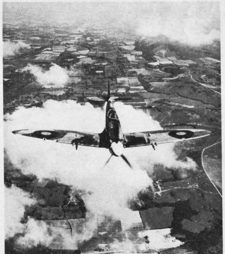
High altitude is the specialty of the new Spitfire—its service ceiling is over 40,000 feet, rate of climb higher than that of previous models.
